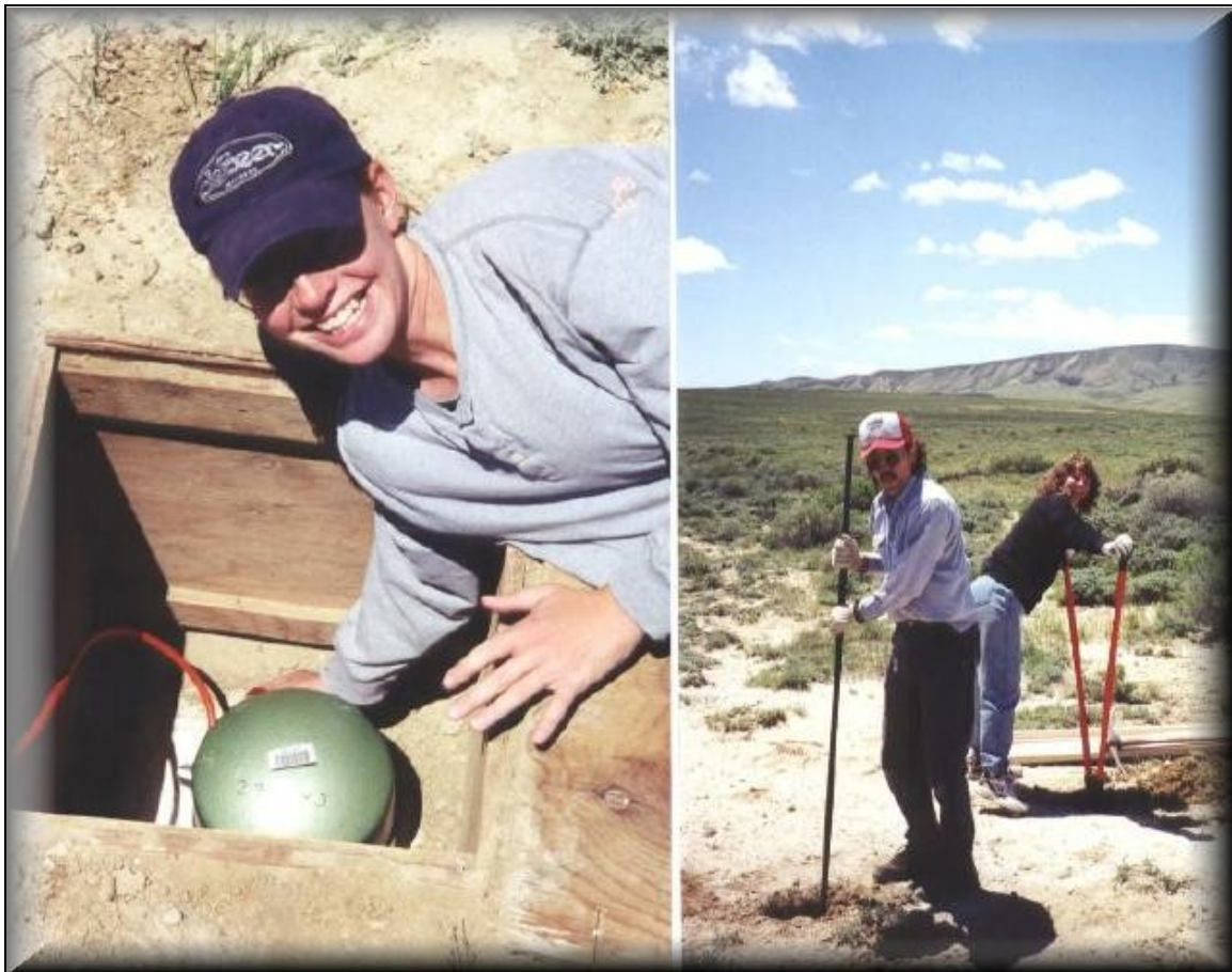
Figure 6. Lynda Lastowka (left) orients a Streckeisen STS-2 in a vault. At the bottom of the vault is the white ceramic tile with an east arrow drawn for orienting purposes. Instrument specialists from the PASSCAL Instrument Center in Socorro, New Mexico help dig post holes for solar panel stands near Rawlins, Wyoming.
